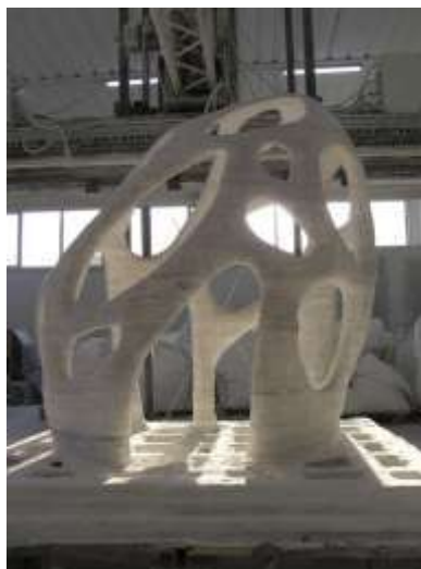
Figura 4.12 - A Radiolaria, impressa na máquina de Enrico Dini, exemplo de D-shape Fonte - https://3dprintingindustry.com/news/robotic-construction-exploring-limits-3d-printing-enrico-dini-99977
